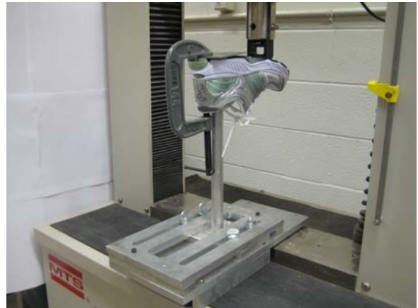
Figure 1: Testing rig with adjustable base and experimental setup in the MTS machine
